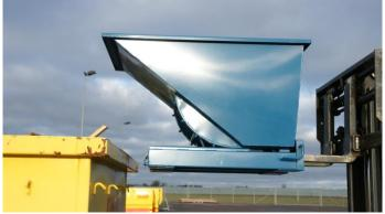
Step 3. Empty the skip automatically (left picture) or manually (right picture)
