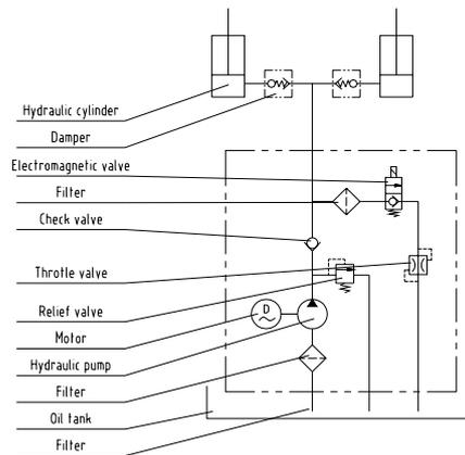
**Fig. 1** Hydraulic circuit
