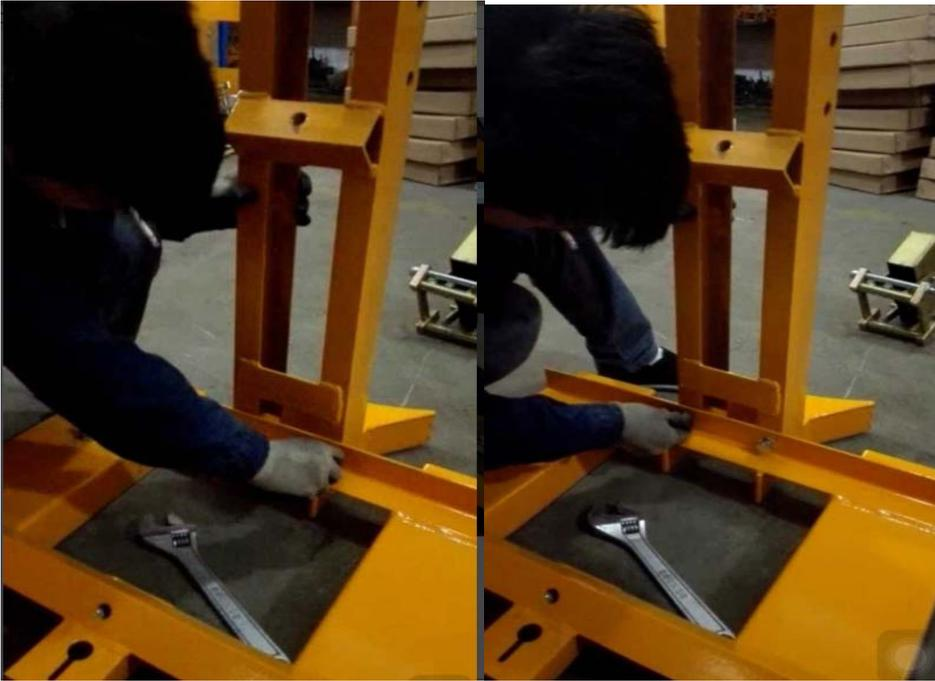
2/fix the connection rod(Y6) on the frame, use parts Y12 Y13 Y14:
