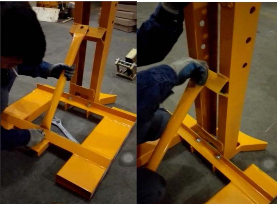
3/take out the fixed pin(Y2) then install the clamps(Y1)on the frame(Y5),use the fixed pin(Y2).At last, use the washer and R shape pin(Y3,Y4) to fix:
