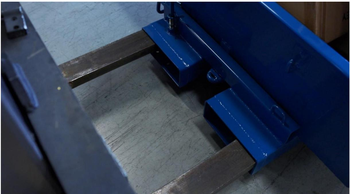
3. Tighten the built-in fork locking for safe handling.
