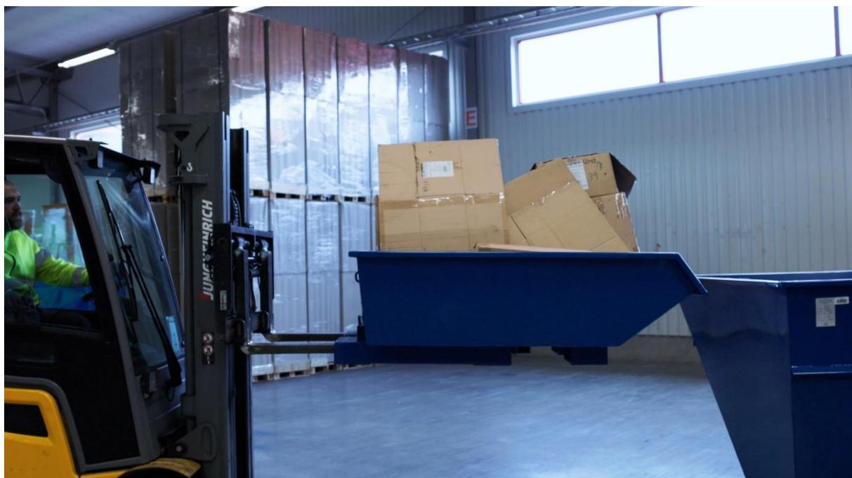
5. Drive carefully towards the edge of the container you are emptying into. Lower the tilting skip over the edge.
