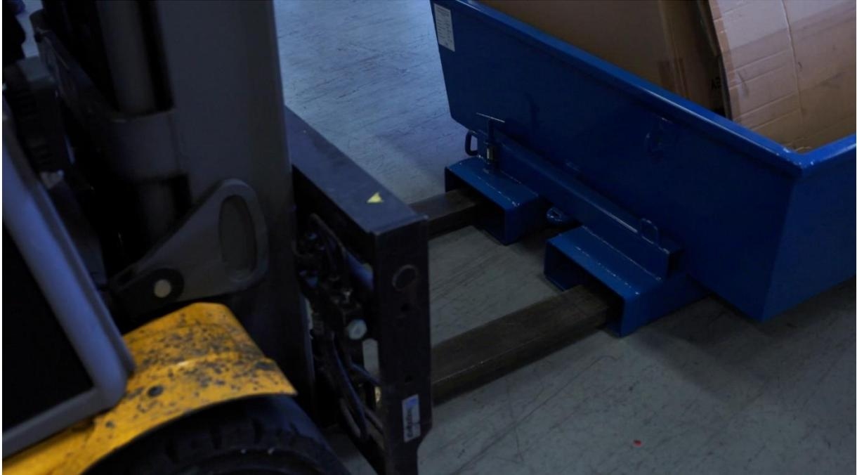
2. Spread the forks outward so that the forks clamp.
