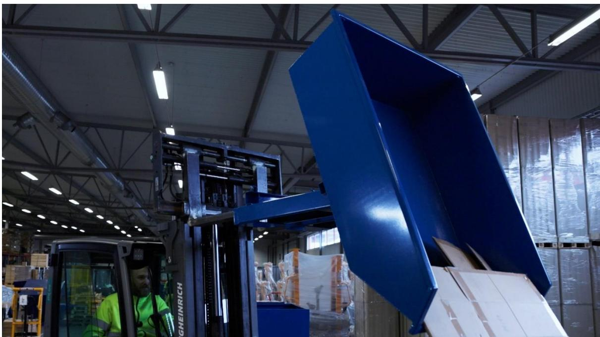
9. When empty, lift it back and lower it to the ground while slowly driving backwards so that the bin tilts back on the undercarriage again.
