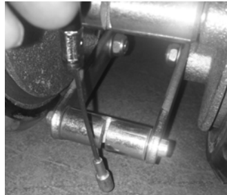
Fig.12: Progressive drive and parking brake
