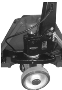
Fig.12: Progressive drive and parking brake
