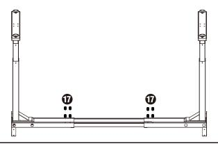
I. Double-check that the base is centered on the underside of the desktop and is located where you want it. Also, double-check that the included wood screws are not too long for your desktop and won't puncture the surface when screwed all the way in.
